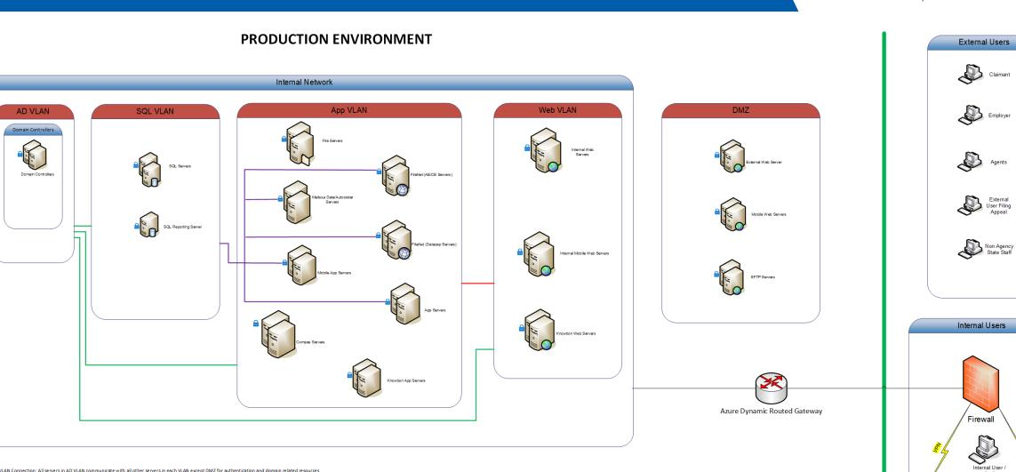
WEB VLAN Connection: Web Servers in WEB VLAN communicate with only with APP servers in APP VLAN
